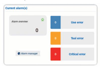
The alarm section allows you to view the history of all errors that have occurred on the tool, whether acknowledged or not.
